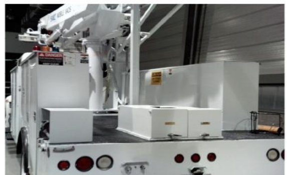
Rear of Vehicle - After Rust Bullet Application
