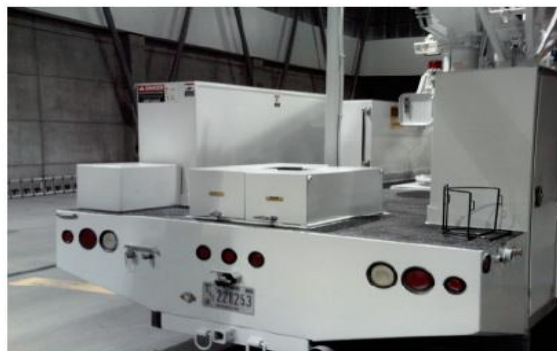
Rear of Vehicle - After Rust Bullet Application
